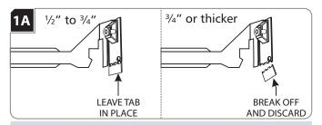
**NOTE:** Skip this section if installing the housing with butterfly brackets.
